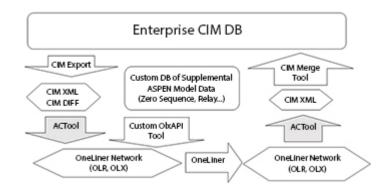
The ASPEN-CIM module will be shipped with a service component, which is designed to help users make custom adaptations to the ACTool to match their existing enterprise CIM profile and also to make it an integrated element in the enterprise CIM data flow.
